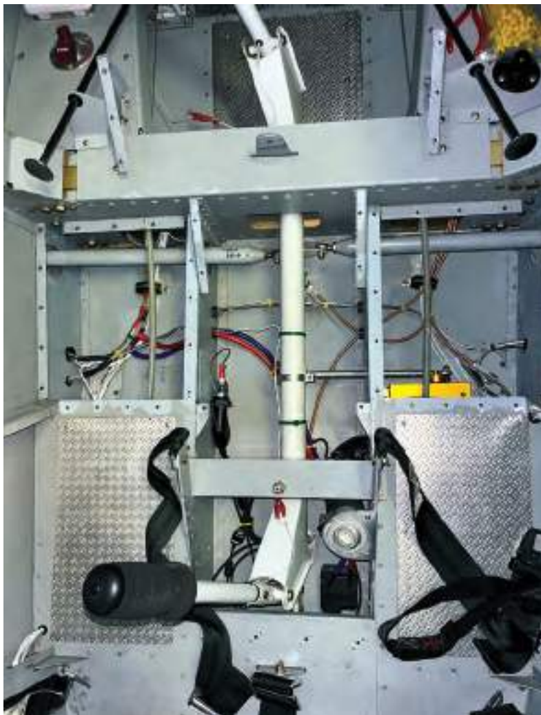
Above Trio Ez-Pilot autopilot hardware install and wiring.
