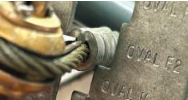
Above Gauge showing under-crimped swage.
