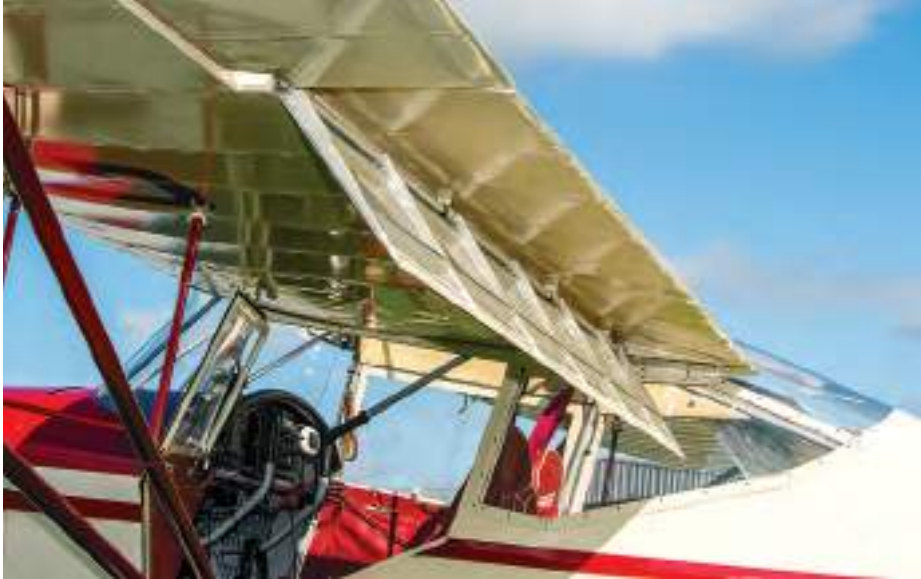
Above Split flaps were built into the Auster AOP6 wings, that were fitted to G-AJIT.
