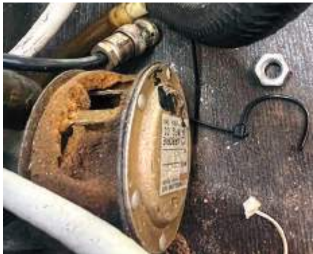
Above Vacuum system filters are not 'fit and forget' items!
