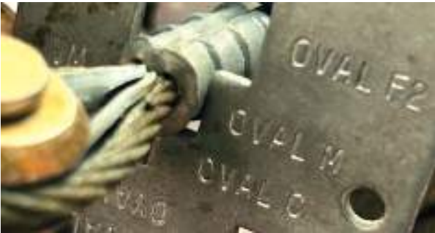
Above Gauge showing correctly crimped swage.
